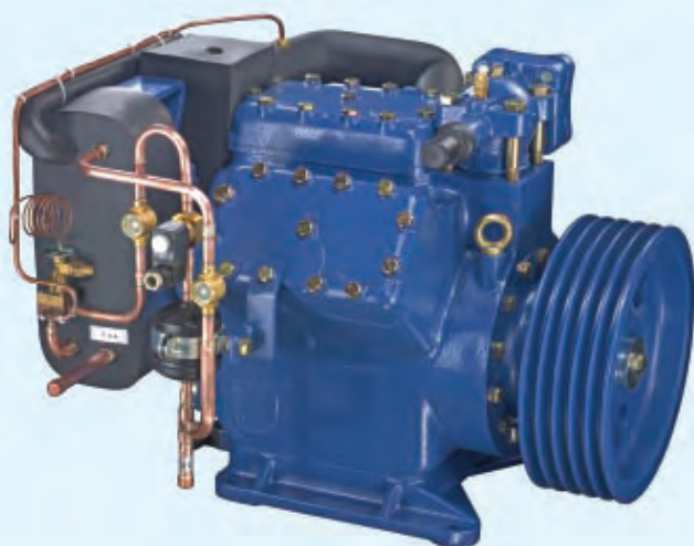
Liquid supercooler, expansion valve, solenoid valve, two sightglasses, filter dryer attached directly to the compressor , lined and insulated.
